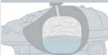
The balance between heating power and boiler pressure and the 1.8 litres steam dome ensure a high quality dry steam.
